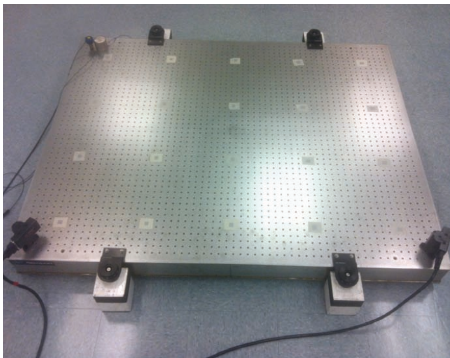
Figure 1. Optical breadboard with add-on active dampers prepared for laser Doppler vibrometer test.
